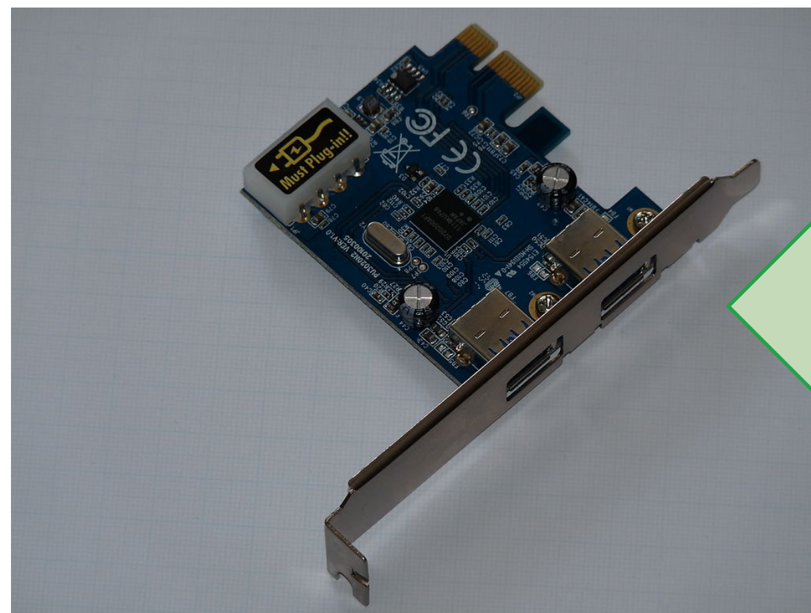
PCIe card with two USB_3.0 ports, 2013, photo courtesy of Dmitry G under public domain
