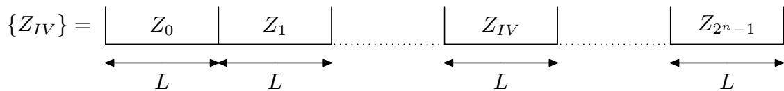
Fig. 2. Exponentially long sequence with direct access associated to an IV-dependent stream cipher g
